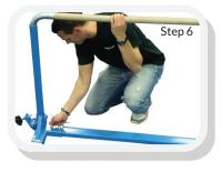
Step 6- Once the bar assembly is seated all the way in the upright, finish tightening the screws in the center support. Repeat for second bar & upright set.
